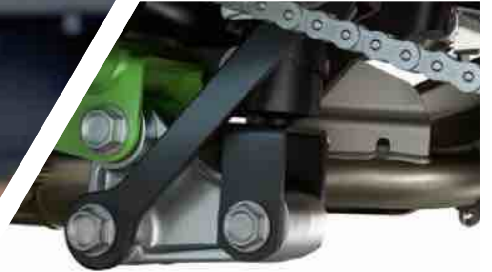
UNI TRAK REAR SUSPENSION FOR GREAT ROAD HOLDING ABILITY AND BUMP ABSORPTION
