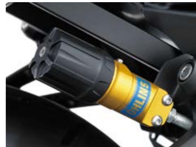
ÖHLINS TTX39 REAR SHOCK WITH PIGGYBACK RESERVOIR AND REMOTE PRELOAD ADJUSTER.*
