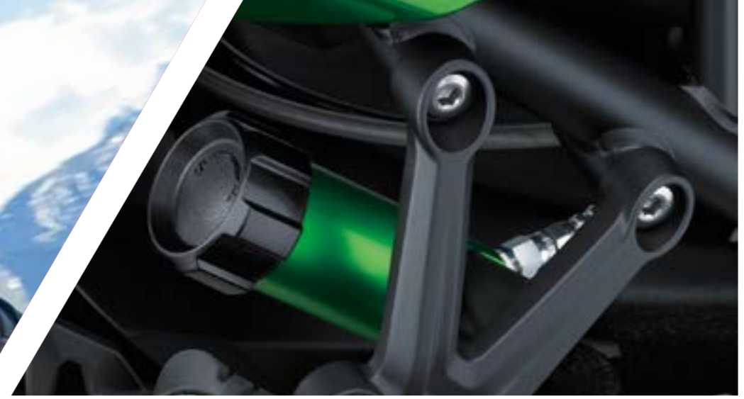
PRE LOAD ADJUSTER ACCOMMODATES FOR EXTRA WEIGHT LOADING
